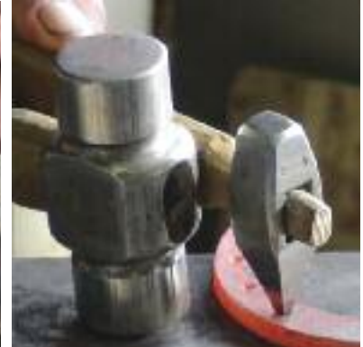
Use hammer to position forepunch to minimize heat build-up in tip. Establish your nail position and punch almost to finish depth.
