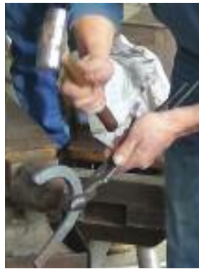
Turn branch over horn, striking the shoe just past the center of the horn to make the bend.
