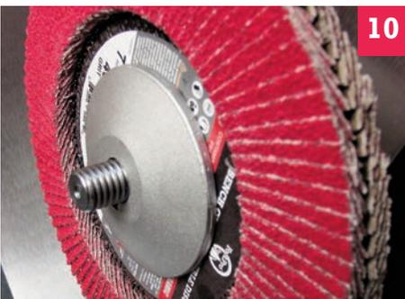
**10** Slide second flange onto shaft and against the disc.
