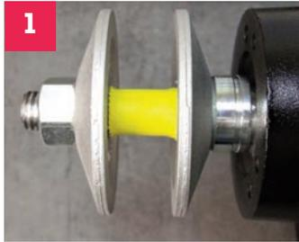
**1** Left side shaft of Baldor 1/2hp out of the box. Shaft is 5/8" diameter and 3.25" long and will require a spacer approximately 1" long. The discs will only fit on shafts that are 5/8" diameter. If you have shorter shafts you may not require a 1" spacer but will likely need a spacer of some length to secure safely.
