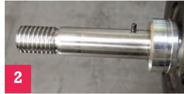
**2** Out of the box, the baldor has a pin in the shaft to hold a flange in place. This will need to be removed before installation.
