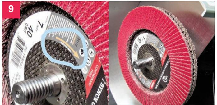
**9** **Be sure you have the rotation correct.** Failure to mount it for the right direction will likely cause damage to the disc and risk of injury. You can mount it on either side of your grinder but it must still be mounted in the right direction.
