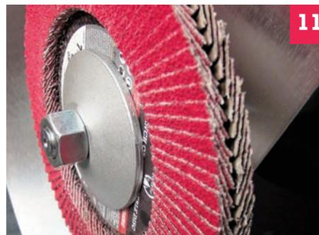
**11** Put the shaft nut on and tighten. Remember that the threads on the left side of a grinder are left hand threads.
