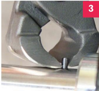
**3** Using a nail cutter, squeeze with just enough pressure to be able to roll the cutter back and pull the pin out. Do not cut the pin.
