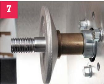
**7** Slide the flange that came with the Baldor grinder on the shaft.
