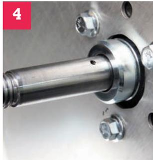
**4** Pin removed. The pin hole may have a slight burr that needs to be removed.
