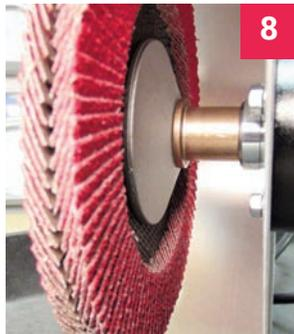
**8** Slide your disc on the shaft. It has a 5/8" arbor so it needs nothing to keep it centered on the 5/8" shaft.
